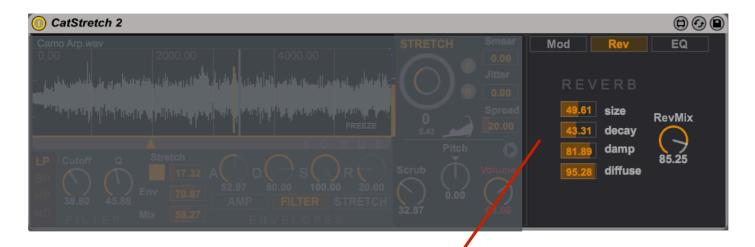
Build-in algorithmic Reverb with Roomsize, Decay, Dampling and Diffusion. RevMix blends between the Dry and the Wet signal
