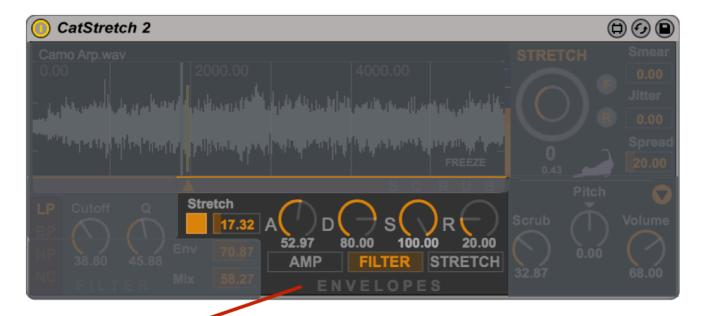
Envelope Section: 3 individual ADSR Envelopes for Filter, Stretch and Volume (Amp). The Stretch Envelope can be switched On/Off and has an Amount switch (similar to the Filter Envelope)
